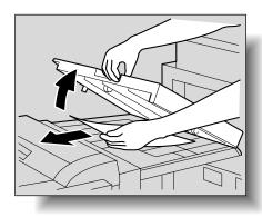
4 Open the feed guide for the finisher, and then remove any misfed paper.
